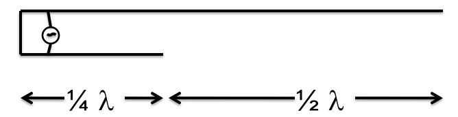
This is a half-wave antenna fed with a quarter wave stub.
