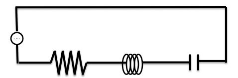
Because charge is accumulating at the ends of the antenna, there is capacitance at the feed point:
